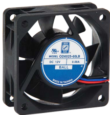
OD6025-60LB Series 60mm x 25mm (2.36" x 1.0") Airflow: 26 CFM
