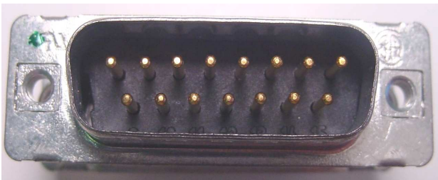
Shell Size 2 15 position Standard 2 row pictured
