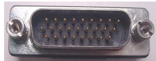
Shell Size 2 26 position High Density 3 row pictured
