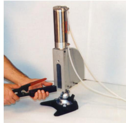
5. Position the hand tool into the bottom center channel of the Power Crimper with the moving half of the crimp tool handle facing up towards the roller above it. Make sure you insert the hand tool far enough into the channel so the ratchet of the hand tool goes through its complete re-opening cycle and allows the crimp jaws to fully open.
