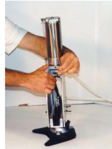
7. Some tools have excessively heavy handles or weak return springs which do not fully reopen the tool and its ratchet. To compensate for this we have provided a return spring attached to the top of the air cylinder. This spring must be hooked by a cable tie or other means to the end of tool handle to insure full reopening of the tool and release of the ratchet.
