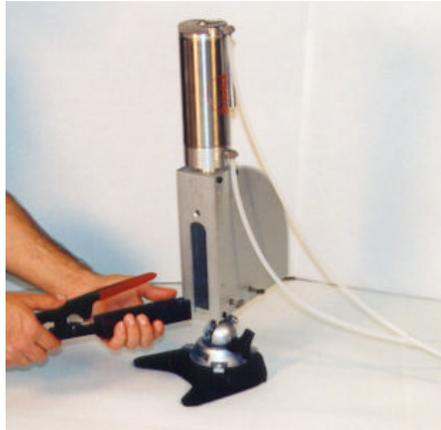
9. Insert the hand tool into its adapter, which is polarized to accept the tool.
