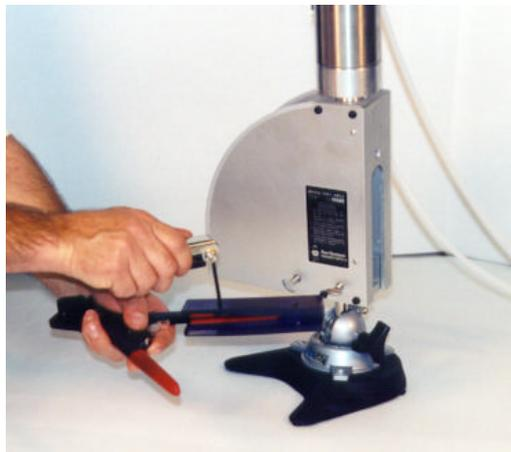
10. Tighten the Allen set screws evenly from both sides of adapter against the tool handle to hold tool securely. Over tightening set screws may distort the adapter, making it difficult to slide into tool channel. Upon completion of this step, follow
