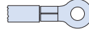
Small Ring for Attaching Receptacle Covers to a Panel with a Screw
