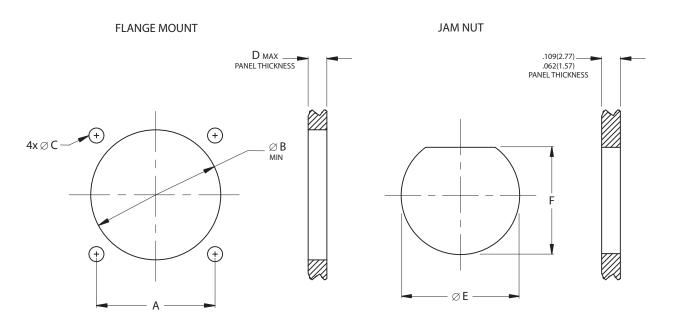
**Note 1:** Flange Mounting Dimensions ( $\varnothing$  B cutout and D MAX) listed only for back of panel mounting (MS27497 and MS27508).
