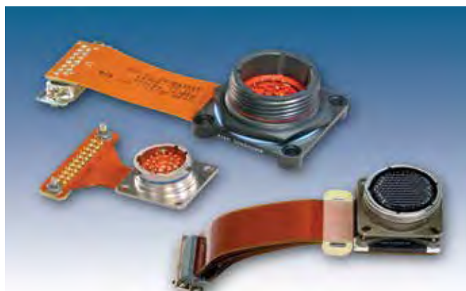
Flex Termination for Attachment to PC Boards
